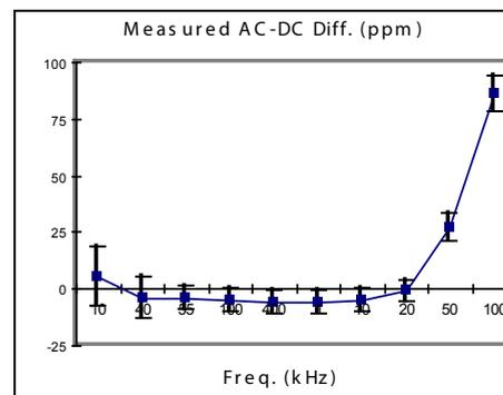
Figure 3. Measured AC-DC difference up to 100 kHz.
