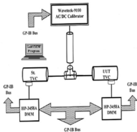
Figure 4. A simplified schematic of the automated measuring system at NIS
