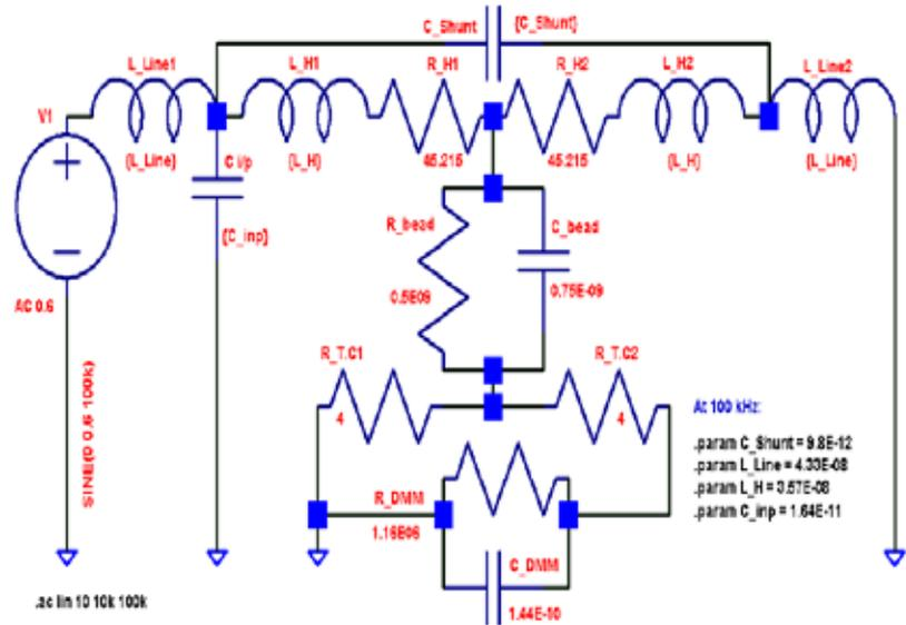
Figure 2. Lumped-parameter model of SJTVC.
