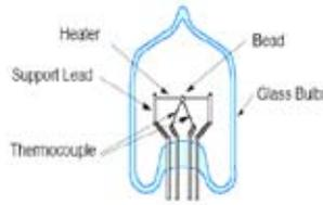
Figure 1. Physical structure of a single junction thermal voltage converter.
